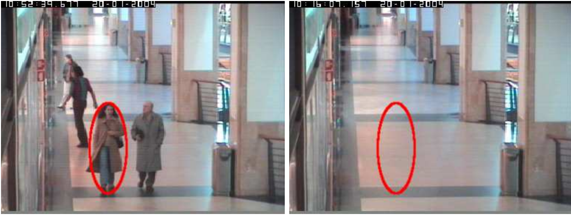
Figure 5.1: A candidate region (left) should be similar in appearance to the object model, but dissimilar to the corresponding region in the background model (right)
