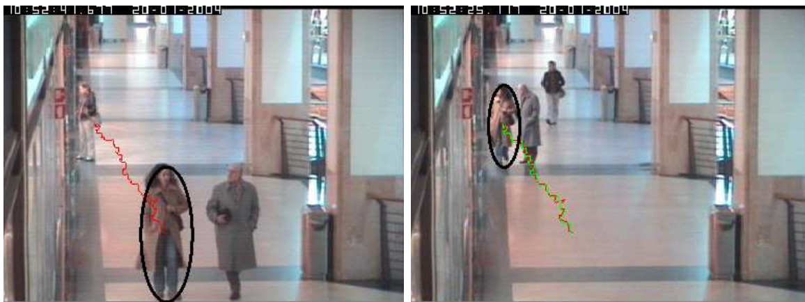
Figure 7.3: An instance of successful track validation (using the gradient-based NCC tracker). The forwards trajectory (red, left) and the backwards trajectory (green, right) for scenario 2 match very closely.
