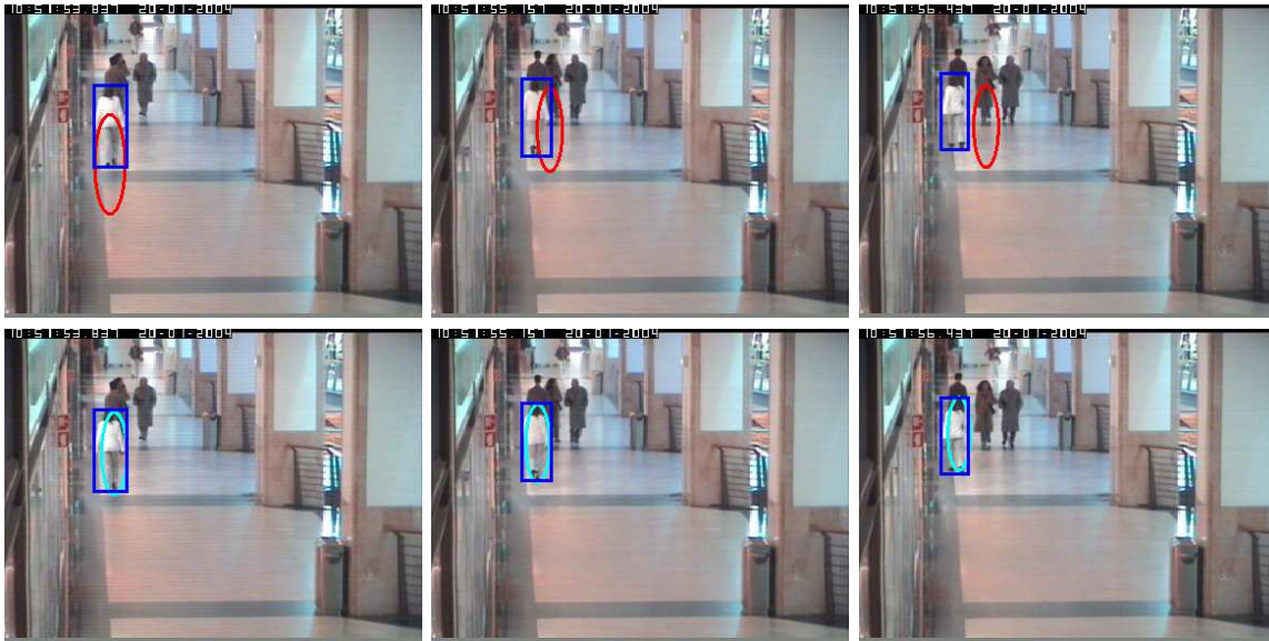
Figure 4.4: Mean shift losing its target (top), while normalised cross-correlation successfully tracks the person (bottom), in scenario 3
