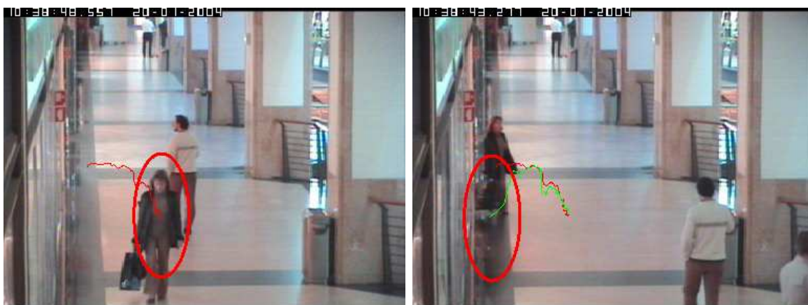
Figure 7.4: An instance where tracking is not validated (using the mean-shift tracker). The forwards trajectory (red, left) and the backwards trajectory (green, right) for scenario 5 are very different.
