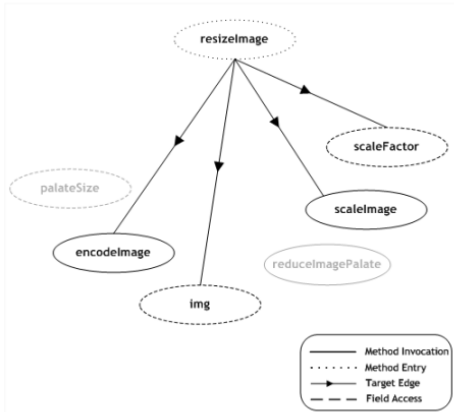
Figure 3.3: An example member dependence graph for a method entitled resizeImage . The graph shows the different types of dependencies that can exist between a method, and other class members. The members that are shaded out, are other class members which are not dependees of the resizeImage method. Local members are not included in the member dependence graph.
