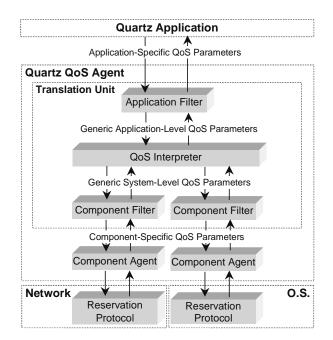
Figure 2. Detailed structure of the QoS agent
