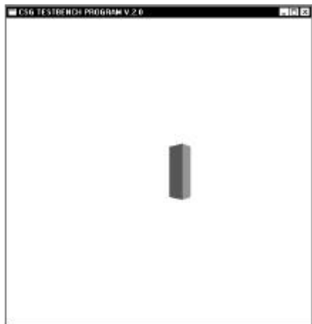
qAND operation draws the intersection of two cubes. The cubes were both rotated by 20 degrees about the Y-axis to produce the “wedge” shape shown.
