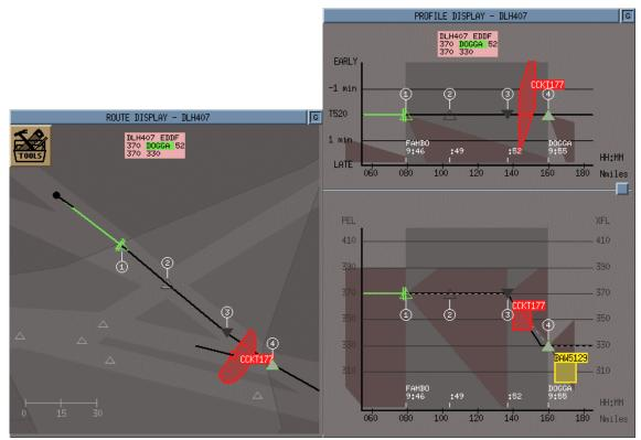
Figure 2: The horizontal, vertical and speed views in HIPS
