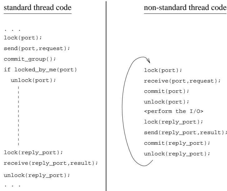
Figure 7.37: An I/O operation development for the second implementation proposal
