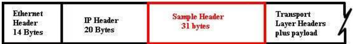
Figure 4.2: SAMPLE header is placed between the IP and Transport Layers
