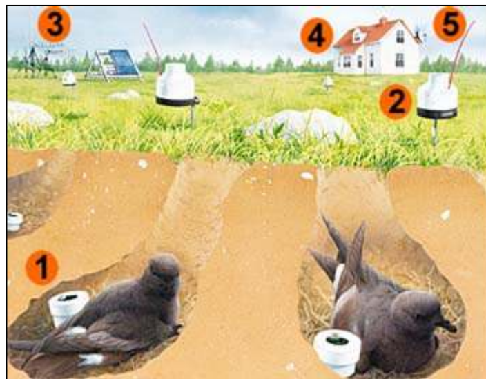
Figure 2.2: Wireless Sensor Network in the Great Duck Island, monitoring the storm petrel (seabird). From 1 to 5 it indicates the process of transmitting data from the motes to the gateway and finally to the satellite [10].
