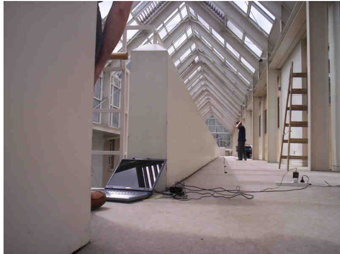
Fig 26 The base station to the left, the ad-hoc network and the person acting as a pedestrian carrying a beacon
