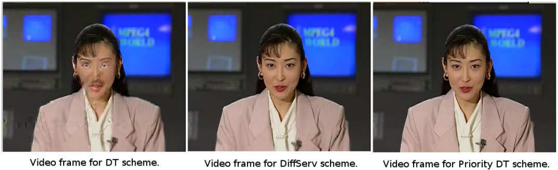
Figure 7.2: Comparison of frame image quality produced by each AQM scheme for video streamed to a client at 300m using the maximum C/I scheduler.
