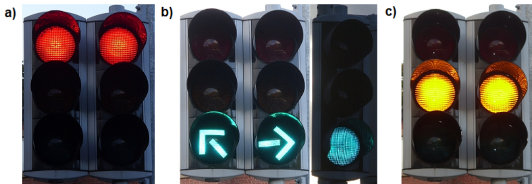
Figure 2.1: Full Irish traffic light cycle: From red directly to green and then, after the split time is over, it changes to amber.
