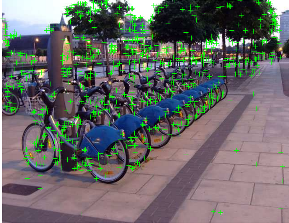
FIGURE 3.7: Sample image P(205).jpg after reject low contrast and edge keypoints (1007 keypoints).
