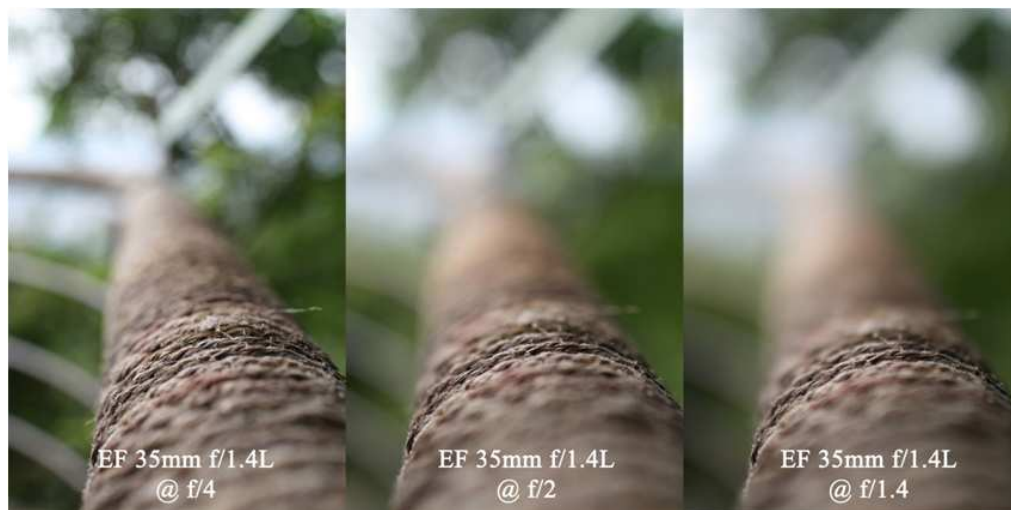
FIGURE 3.20: Illsion the different size of the aperture cause different depth of field. The image is from edwinsetiawan
