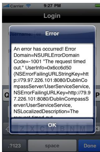
Figure 41 – The outcome of evaluating an Internet-based function which is invoked in a no-Internet environment.
