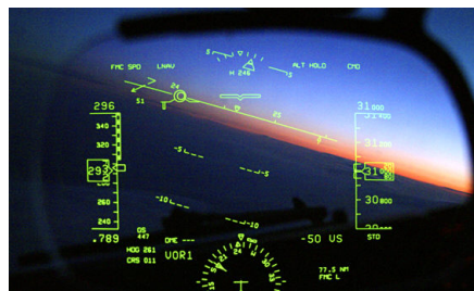
Figure 1.2: The HUD of an aircraft
