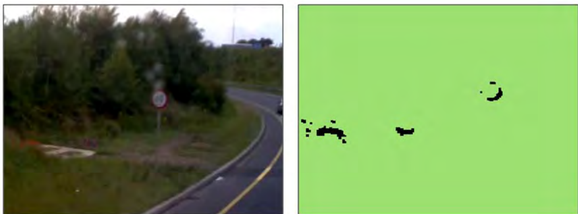
Figure 5-4 A False Negative result was caused by the rain drops on the windshield.
