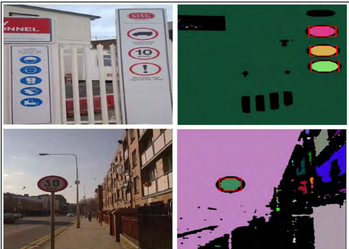
Figure 4-6 Two original images (left) and their labelled region images (right). Non-red ellipses are marked with red rectangles.
