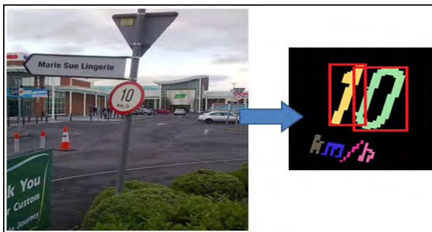
Figure 5-3 A serious sloped speed limit sign causes system misclassified it as a negative sample.
