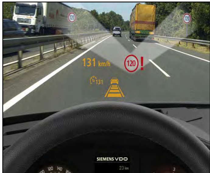
Figure 1-1 Siemens VDO scans the road for speed limit signs and adjusts the speed accordingly.
