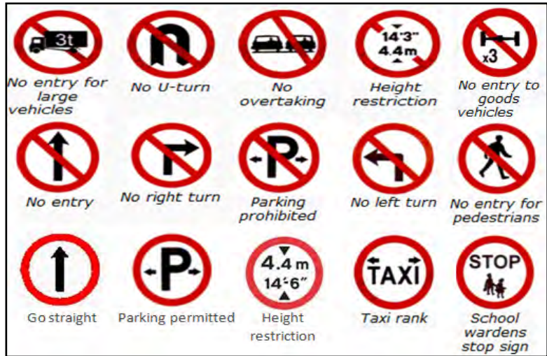
Figure 3-10 After non-red ellipses have been identified, regulatory traffic signs in the first two rows can be eliminated by the system because the ellipses are split into two different regions by the red backlash strip.
