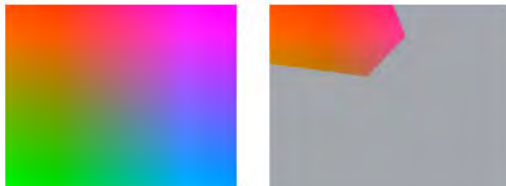
Figure 3-4 Original image (left) and the result (right) after red colour detection.
