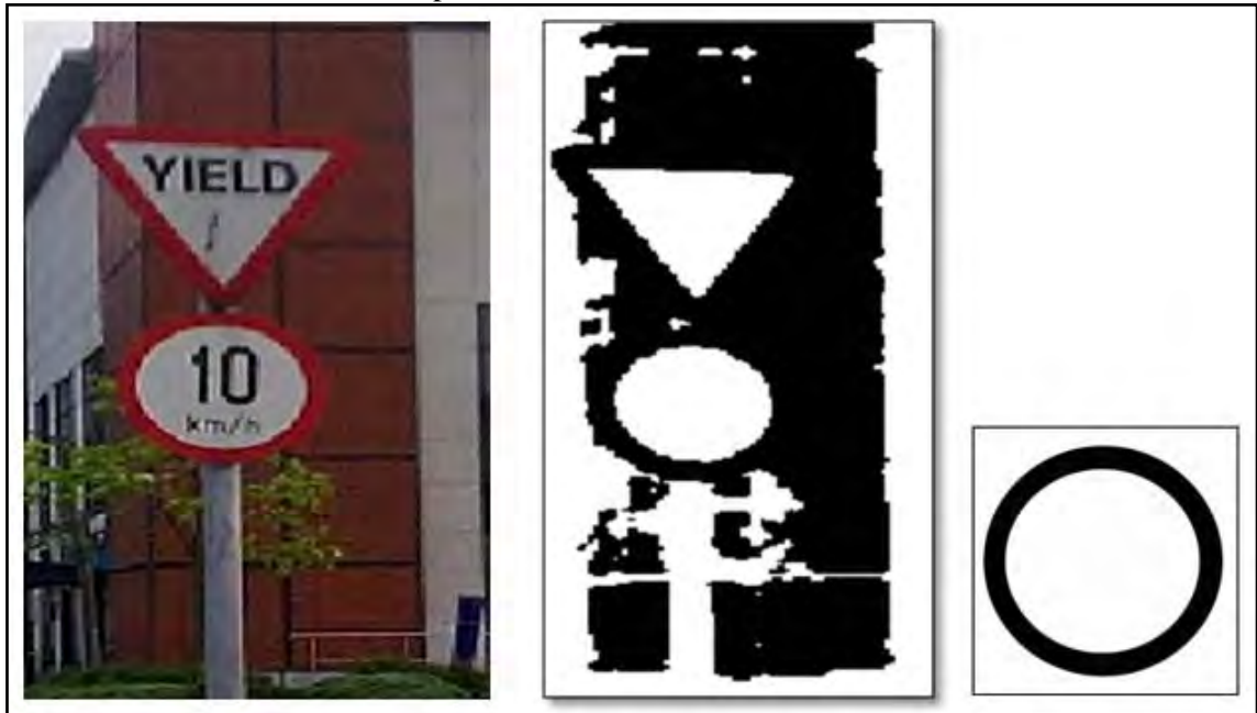
Figure 3-8 Template matching technique could fail to detect red circle surrounds the speed limit sign when the red circle melted into the background red area (from left to right: original image, binary image after red colour extraction and the template image).
