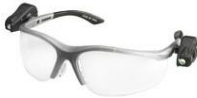
Figure 28 - Glasses used for head tracking with IR LEDs on the sides
