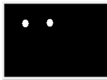
Figure 29 - What the Wii remote sees - the white dots represent the IR light detected
