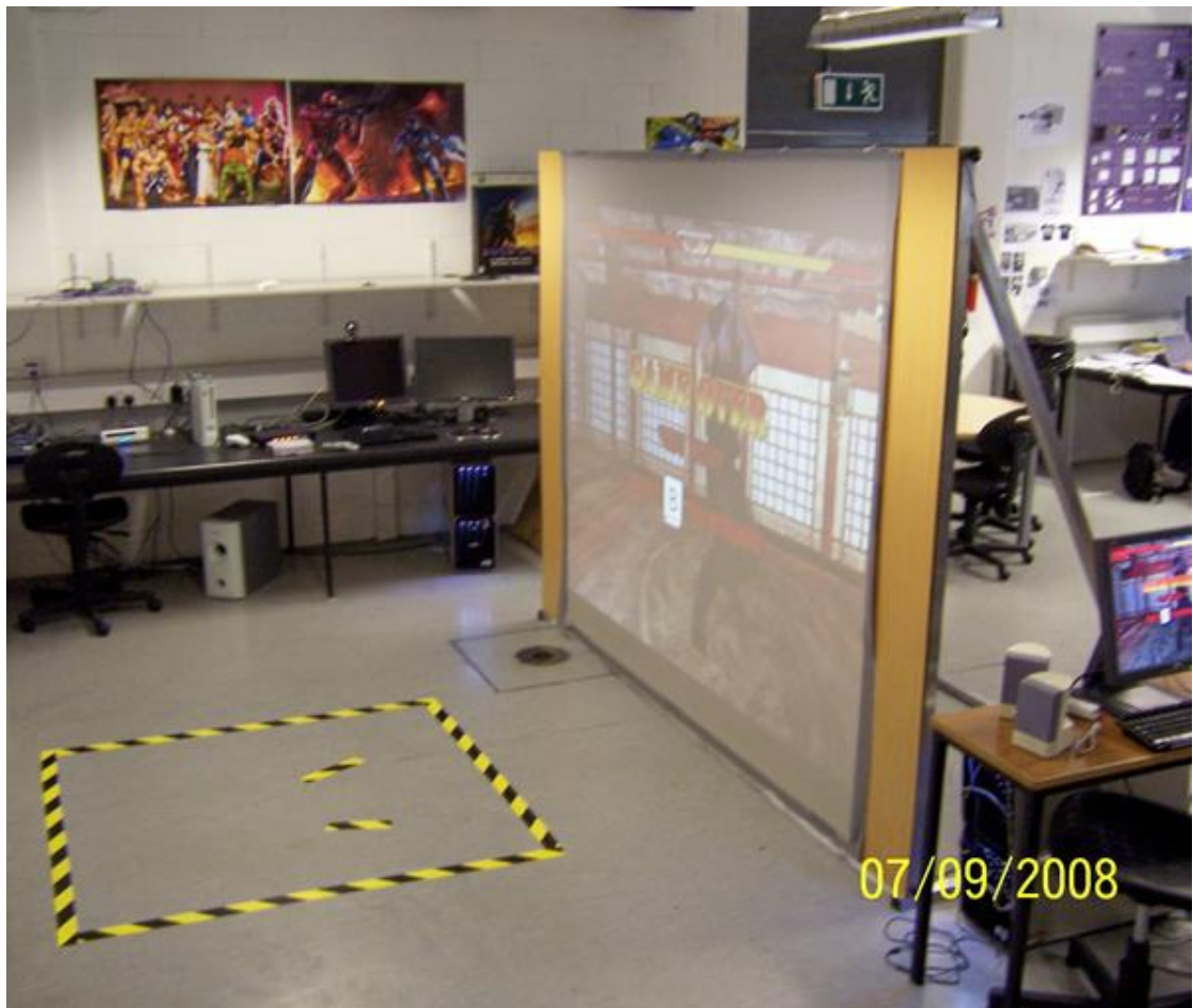
Figure 45 - Entire Kendo Game setup - playing area, screen, USB camera and Wii remote
