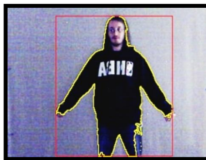
Figure 37 - Body tracking: yellow represents the Freeman chains and red represents the bounding box
