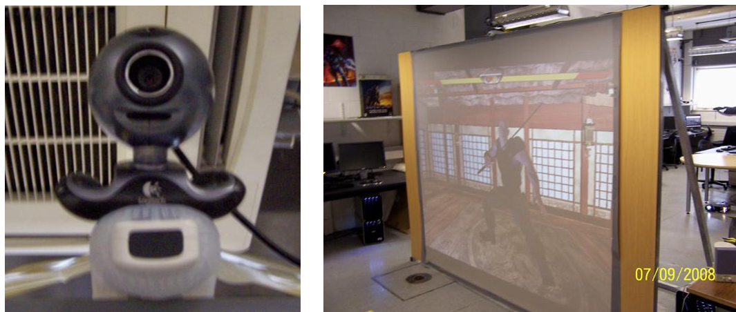
Figure 44 - Close up of USB camera, Wii remote and back projection screen
