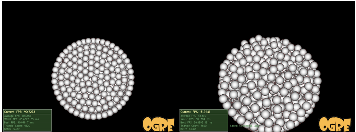
Figure 3.7: A comparison of the surface detail of SPH (left) and of control point SPH (right) at equilibrium. In SPH the particles are spread evenly across the surface due to perfect symmetrical forces but the number of particles at the surface for SPH and control point SPH are relatively the same and so the level of detail obtained when the fluids are in motion is effectively the same.
