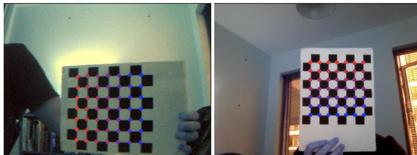
Figure 4.3: Camera Calibration: Feature identification
