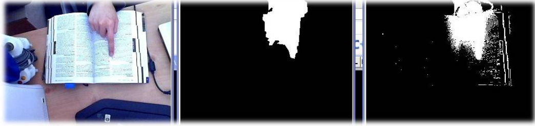
Figure 5.7: From left to right: the current frame captured from webcam; the image after compute the difference between background and current frame; result after connected component operation.
