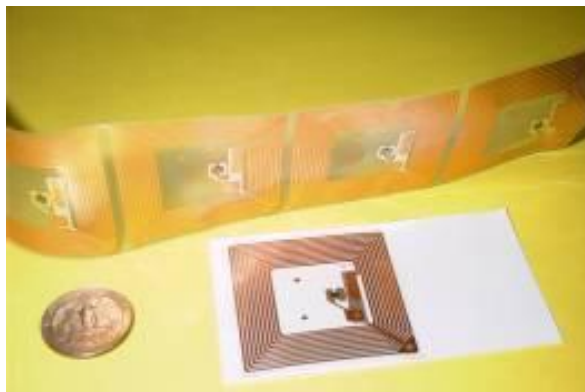
Figure 2.3: RFID transponders (tags). Flexible copper printed onto clear plastic, embedded between two printed sheets to create one page thickness for the Listen Reader books.
