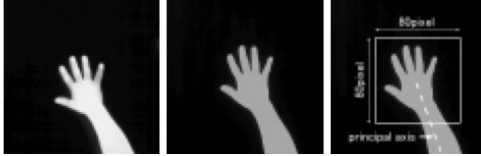
Figure 2.5: Extraction of hand region by an infrared camera.
