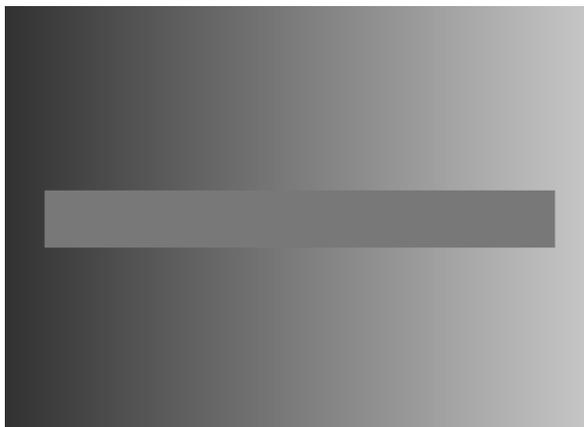
Figure 1.1: A well known optical illusion demonstrating the gradient based method which the human visual system is suggested to use. The grey bar across the middle of the image has a constant intensity, however the varying shade in the background misleads the brain.
