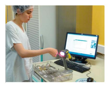
Figure A3; Scanning the DataMatrix 2D barcode on a surgical instrument (Nicolaos et al., 2010)
