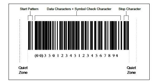
Figure A4; General Format of a GS1-128 Bar Code, (GS1 General Specifications, 2012)
