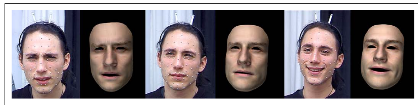
Figure 2.1: Example of passive marker motion capture [14]
