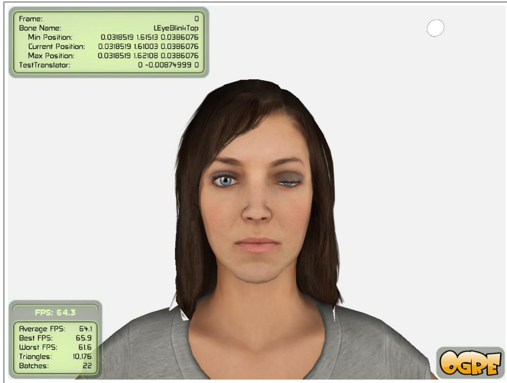
Figure 4.3: Specification process within retargeting application. Top pane provides notable information for bone limit specification
