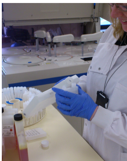
Figure 4.15: Calibrator for each drug type is decanted into an Aliquot which is then placed in the Analyser
