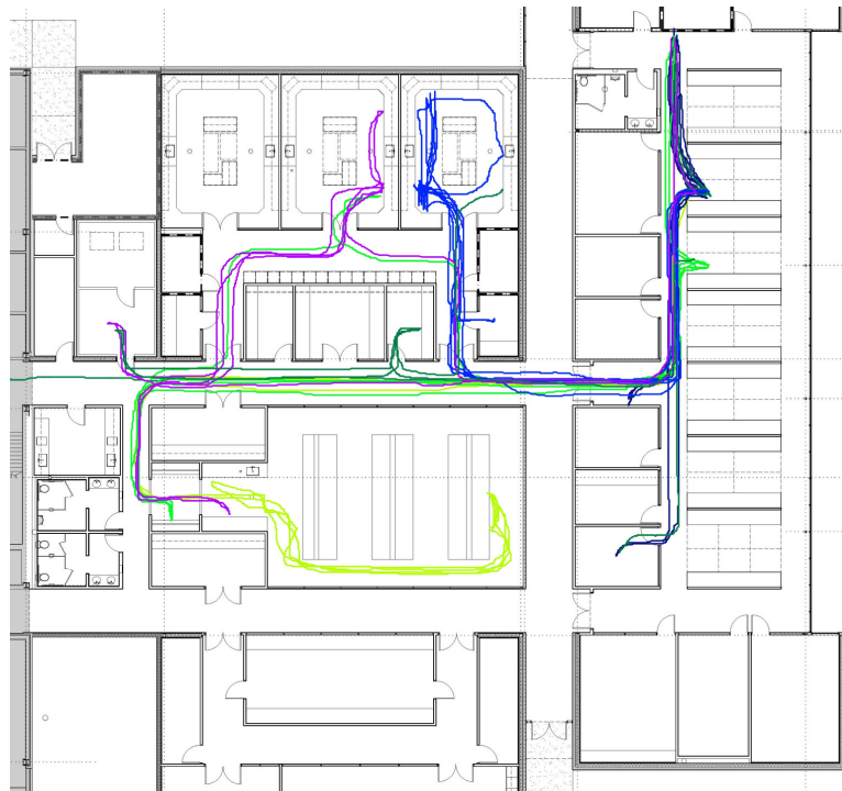
Figure 2.9: This Spaghetti diagram shows the new process flow (approximately 7879 feet or 1.5 miles) the LSS implementation (Richard, Kupferschmid, 2011)
