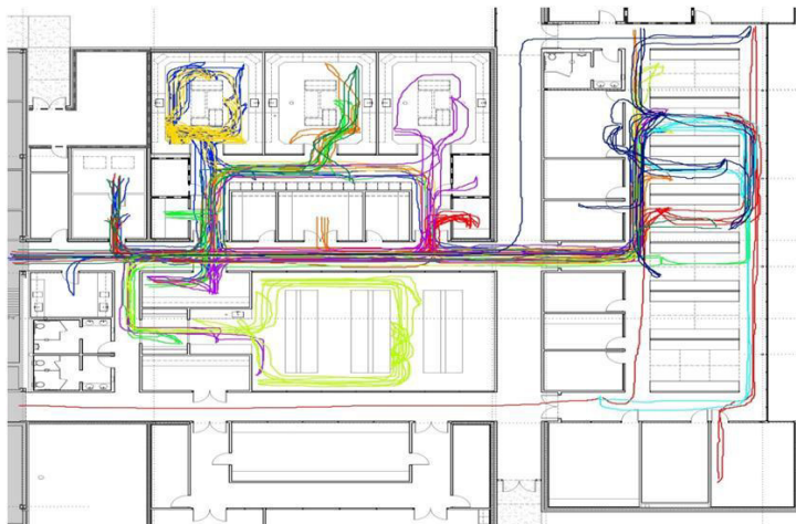
Figure 2.4: Spaghetti diagram showing the steps travelled to complete a process, (Richard, Kupferschmid, 2011)
