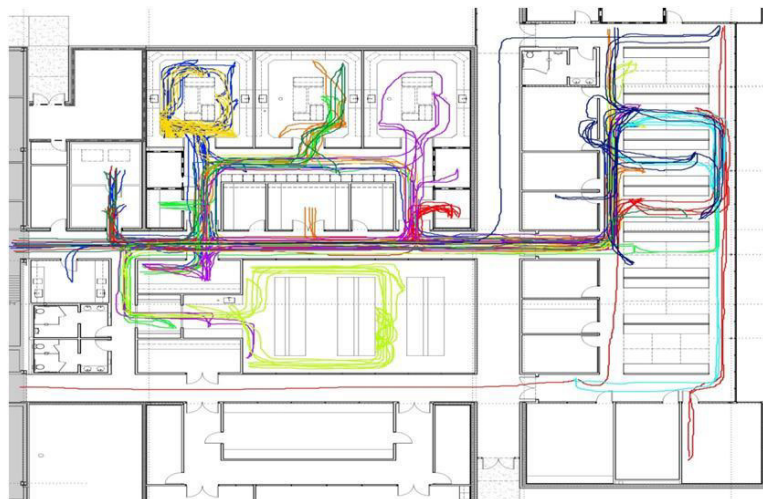
Figure 2.8: This Spaghetti diagram shows the steps travelled (approximately 12,687 feet or 2.4 miles) before the LSS implementation (Richard, Kupferschmid, 2011)
