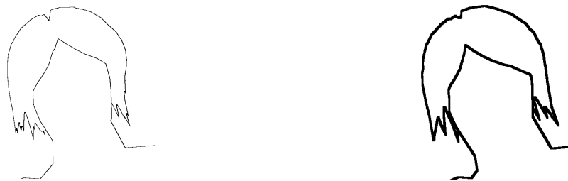
(a) The scene after an edge detection pass. (b) The edge image after a dilation pass.
