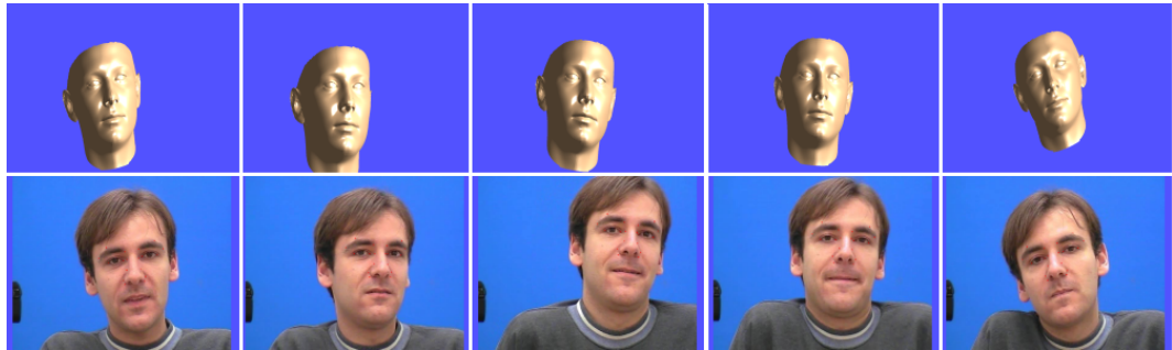
Figure 3.6: The results of the normalised DLT algorithm when it was implemented on Timothy Cootes' video. The bottom row displays the images taken from Timothy Cootes' video. The top row displays results obtained when the algorithm was applied to the data.
