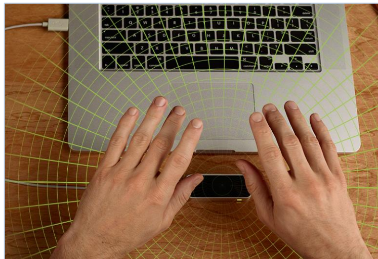
Figure 21 Leap Motion sensor field of view (© 2014, Leap Motion, Inc)
