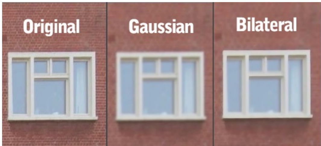
Figure 4.1: Original Image(Left), Gaussian filter(Middle), Bilateral filter(Right). Kernel size 7x7
