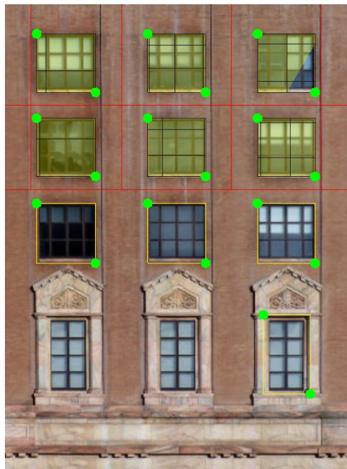
Figure 8: First floor windows were not detected due to additional frame gradient, causing the algorithm set seconds floor as the first one.
