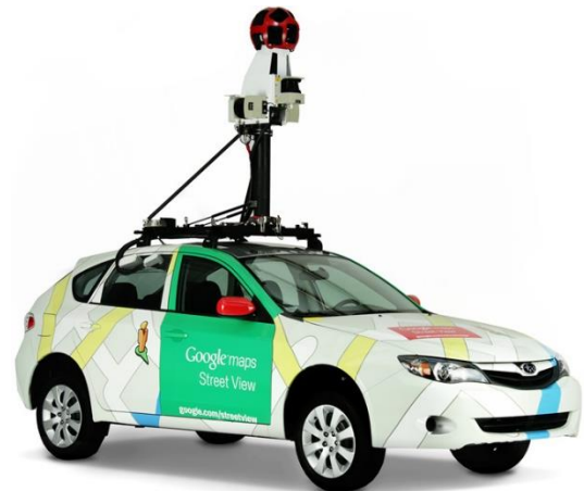
Figure 12 (Google, 2014) An example of a car used by Google to record images for their Street View service. Note the laser sensors and panoramic cameras and the height of the camera
