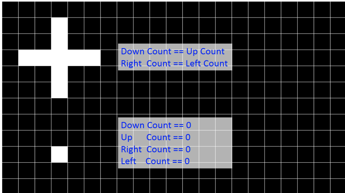
Figure 22 Shows the remaining two scenarios where all counters are equal and the result is a crossroad shape and when all the counters are zero and no cornered shape exists.
