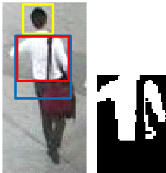
Figure 9: Head detected with yellow box at top, initial and refined estimates in blue and red boxes respectively. Thresholded upper torso region shown on right.
