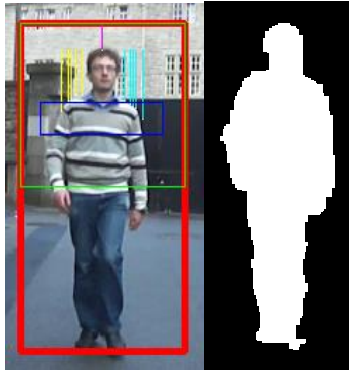
Figure 20: Locating the top of the shoulders using the foreground mask.
