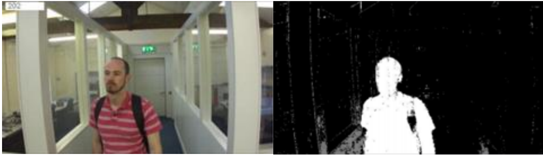
Figure 3: Original image on left, a mask showing the detected foreground regions in white on the right with shadows in grey.
