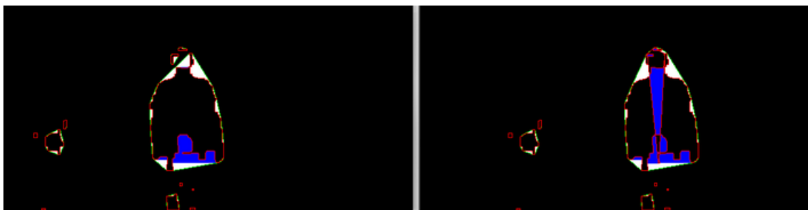
Figure 19: On the left is the original image with filled in regions shown in blue. On the right we can see how the disjoint regions around the head have been combined.
