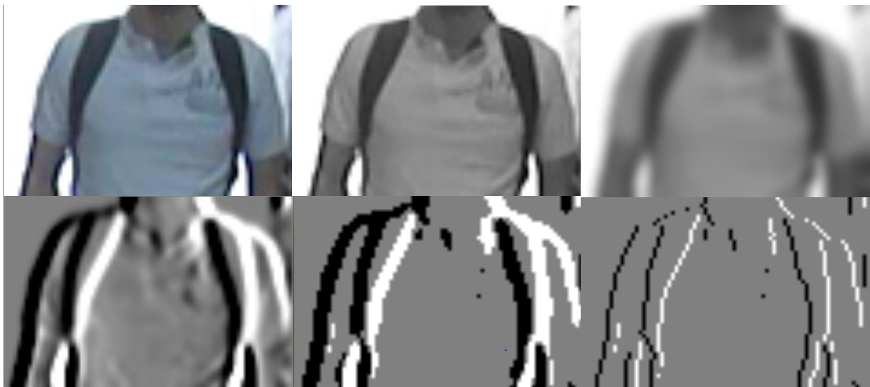
Figure 32: Top Row: Colour Upper Torso Region, Greyscale Upper Torso Region, Gaussian Blurring Applied Middle Row: 1st Derivative Sobel in x-direction, Thresholding applied, Non-Maxima Suppression Applied
