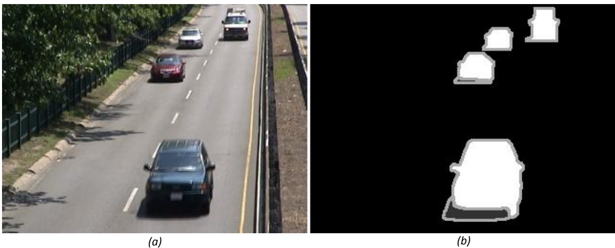
Figure 3.1.5 - (a) Original frame, (b) Corresponding ground truth frame with a variety of labels. Foreground pixels are coloured white, background pixels are black, unknown pixels are light grey and shadow pixels are dark grey (source: [14])
