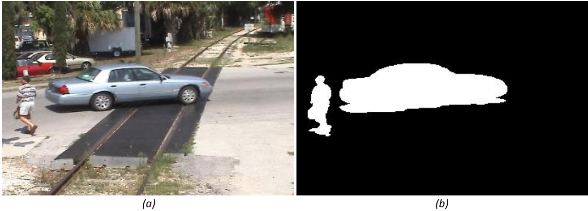
Figure 3.1.4 - (a) Original frame, (b) Corresponding binary ground truth frame. Foreground pixels are coloured white, background pixels are coloured black (source: [47])
