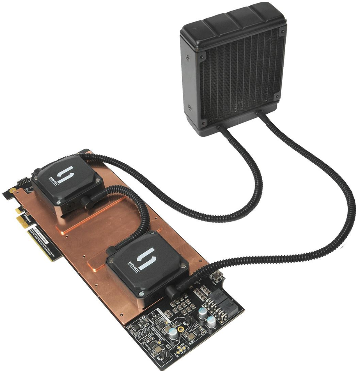
Figure 7 Butterfly Labs Imperial Monarch Mining card & Liquid cooler [16]
