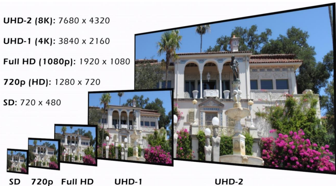
Figure 8: Comparative resolutions of the UHD formats compared to HD and SD TV resolutions
