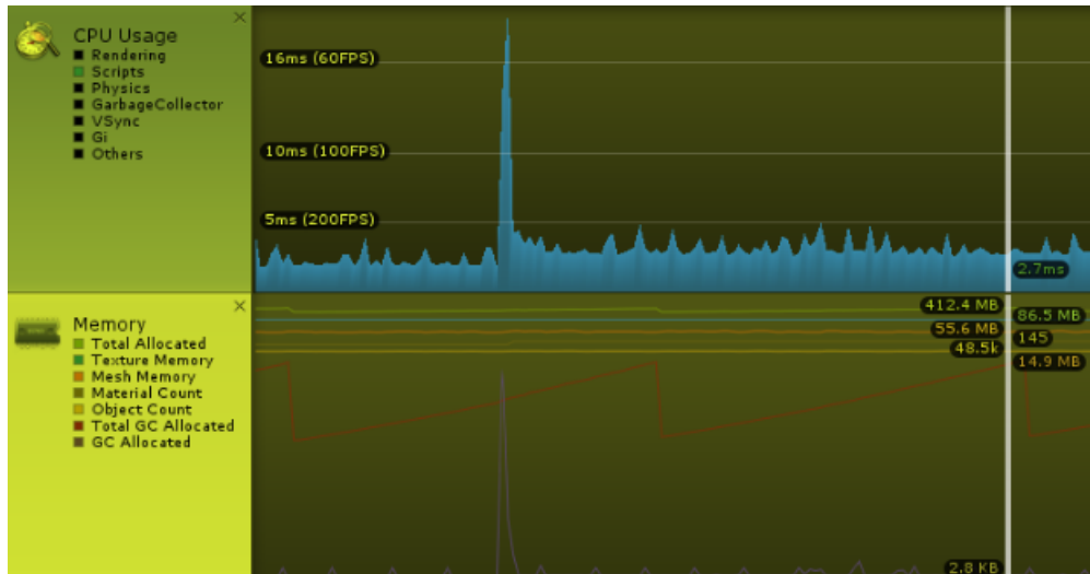
Figure 5.1: Unity’s profiler showing McNulty’s implementation. The performance shows a computation spike, which adversely affects the frame rate. This corresponds to 10am in-game time, when all NPCs go and eat breakfast. Other than this, performance is steady.
