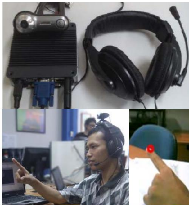
Figure 19: Proposed System. The user can control the application through voice commands or through pointing their finger at the object of interest.
