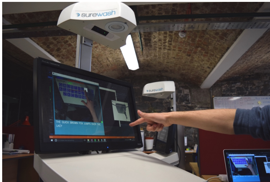
Figure 5.15: A user extends their index finger and thumb to initiate a swipe gesture.
