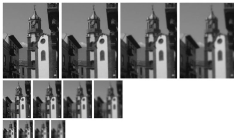
Figure 25 - Three octaves of scale space for the image of a clock tower [13]
