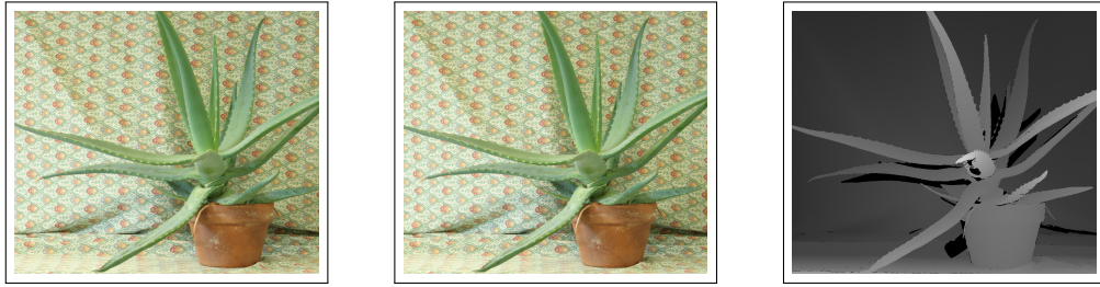
Figure 2.13: Left and right stereo images combined to produce a disparity map. Images were produced for the stereo vision research of Daniel Scharstein, Richard Szeliski and Heiko Hirschmiller [12]
