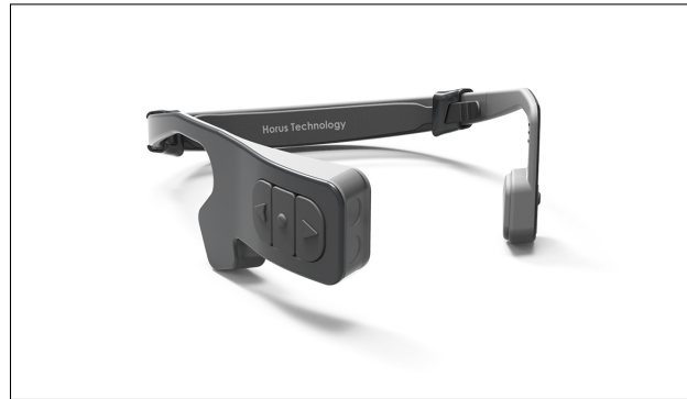
Figure 2.5: Horus Technology headset contains a camera with bone conductors to be placed on the jawbone, just below the ear [5].
