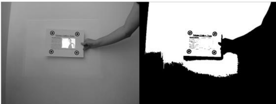
Figure 4-3 Grayscale to binary using Otsu thresholding
