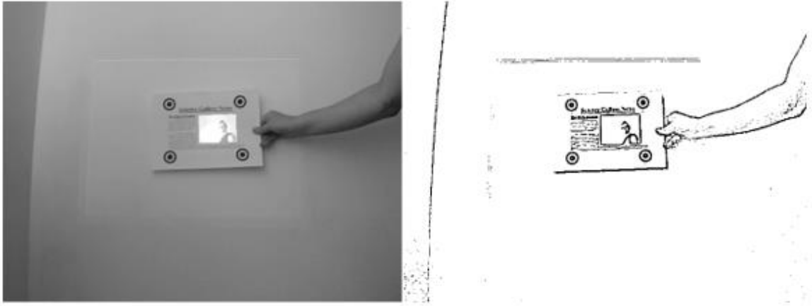
Figure 4-2 Grayscale to binary using adaptive thresholding
