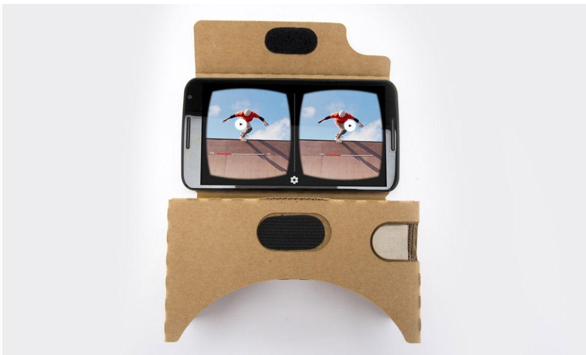
Figure 18: Google Cardboard VR2 with input button and smartphone. Display is split stereoscopically for Google Cardboard lenses (Lang, 2016)
