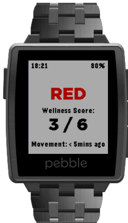
Fig. 5.2. Pebble watch displaying warning yielded for a patient with an increasingly poor outcome.
