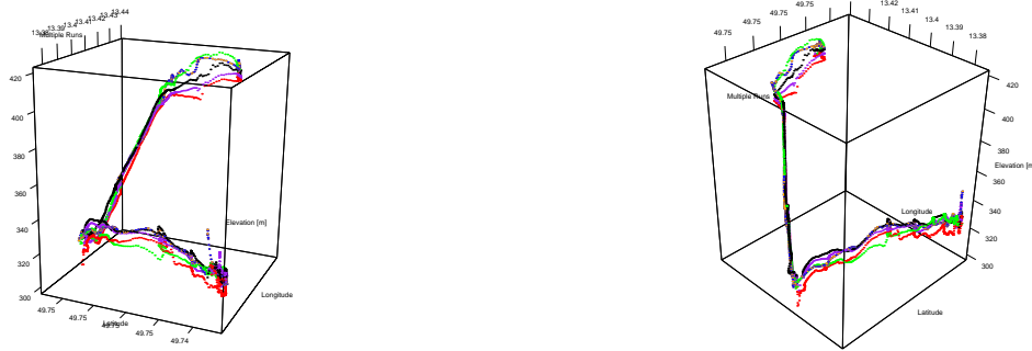
Figure 6.22: 3D representation of five repeated runs of the test segment, the different colours representing each run, comparing the elevation to the longitude and latitude coordinate measurements taken from the GPS module.
