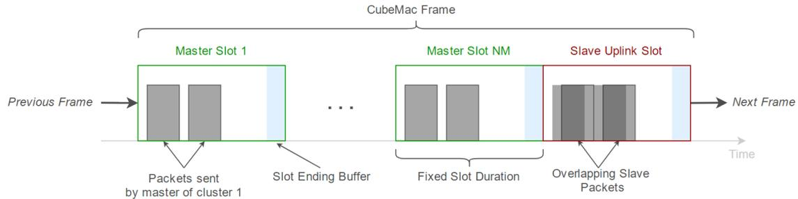
Figure 21. One complete CubeMac frame. “Master Slots” are collision free through TDMA. Communication during “Slave Uplink Slots” is made collision free using CDMA. Frames repeat indefinitely.
