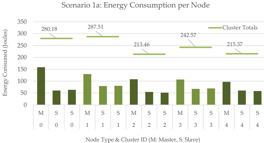
Figure 42. The total energy consumed per node during scenario 1a's simulation run. As masters must handle the routing of all slave packets as well as S2G communications, their energy consumption is notably higher. Masters consumed an average of ~120J and slaves consumed an average of ~64J.
