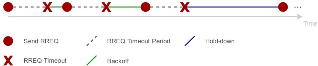
Figure 32. A node attempts three route discoveries by broadcasting an RREQ. In each case the RREQ timeout period elapses before an RREP is received. Following each timeout a back-off period is observed before sending another RREQ. Failing the maximum number of sequential discovery attempts sends a node into a hold-down state
