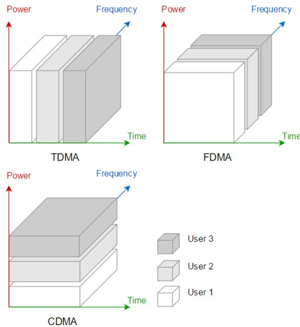
Figure 16. A comparison of common contention free MAC schemes. In CDMA, a 'chip', or code, is used to ensure that signals on the medium are orthogonal and therefore cannot collide.
