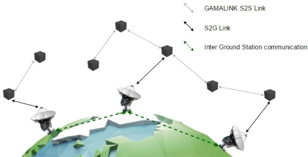
Figure 6. Unlike NASA’s EDSN approach (Figure 2), Gamalink seeks to establish multi-hop CubeSat networks capable of communicating with multiple ground stations. Gamalink designers refer to such networks as GAMANETs.
