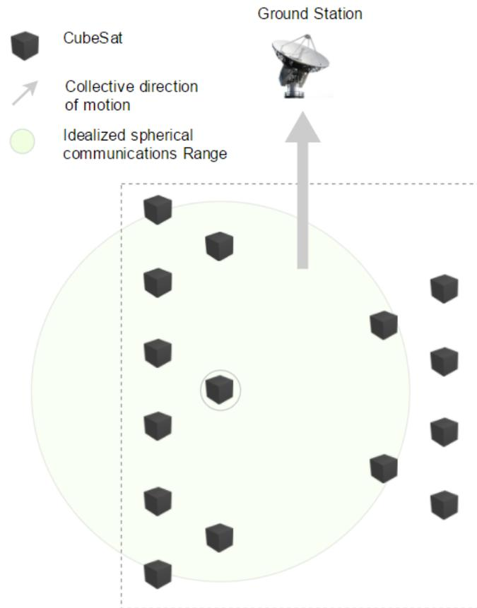
Figure 3. The CubeSats and ground station of the hypothetical as viewed from a higher orbit looking down upon the Earth's surface. The CubeSats are assumed to have an orbital altitude of 550km.
