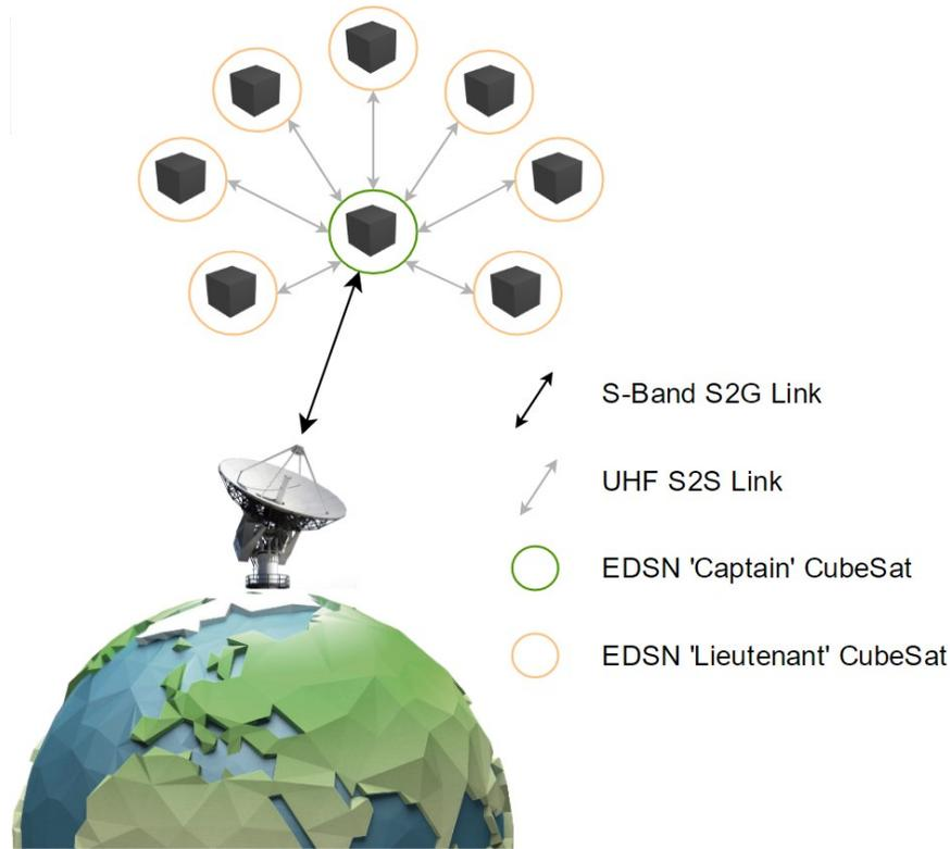
Figure 2. An illustration of EDSN CubeSats in orbit forming a star (hub-and-spoke) topology CSN. Each CubeSat houses two radios, one for S2S the other for S2G communication. Communication to ground is performed only by the current 'Captain' CubeSat.
