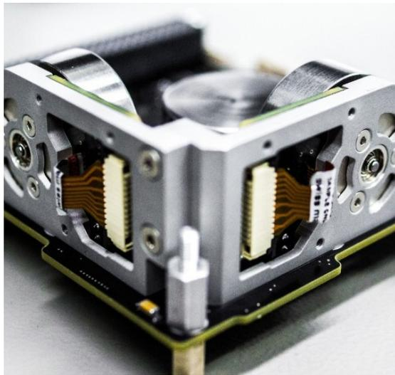
Figure 7. A COTS CubeSat attitude control unit. The rotational velocity of the three reaction wheels shown can be altered to adjust a craft's attitude. Image Credit: Clyde Space Ltd, All Rights Reserved.
