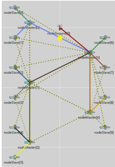
Figure 53. The “early” election of nodeMaster[3] using the energy-distance election approach. The point at which nodeMaster[3] would be elected GM using the closest-master approach is represented by a yellow circle.
