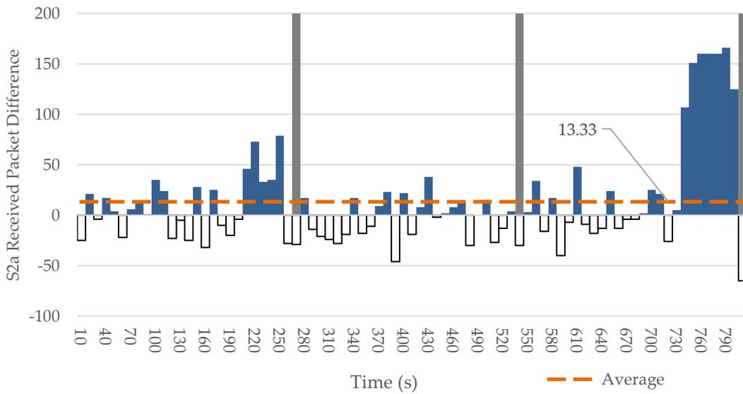
Figure 45. The difference over time in the number of packets received in scenario 2a as compared with scenario 1a. Negative values (outlined) represent interval values in which scenario 1a’s ground station received more packets than scenario 2a’s ground station.
