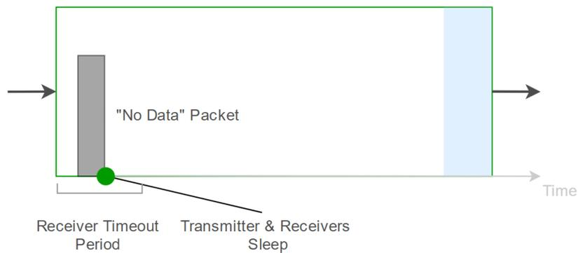
Figure 26. Nodes may generate a “No Data” packet when they have no data to send during their slot. Sending this packet incurs an energy penalty but this may be outweighed by allowing multiple nodes to sleep prior to a timeout.
