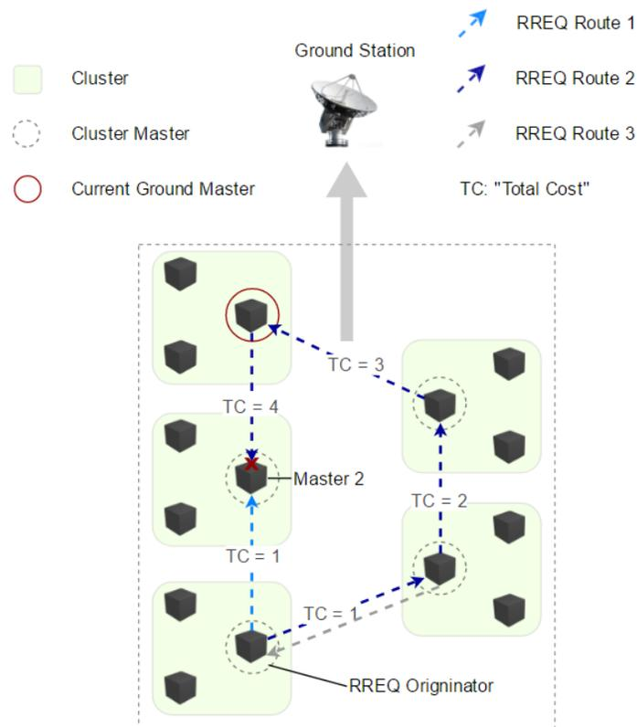
Figure 31. DYMO detects loops by comparing a route message's cost metric with relevant existing route entries.
