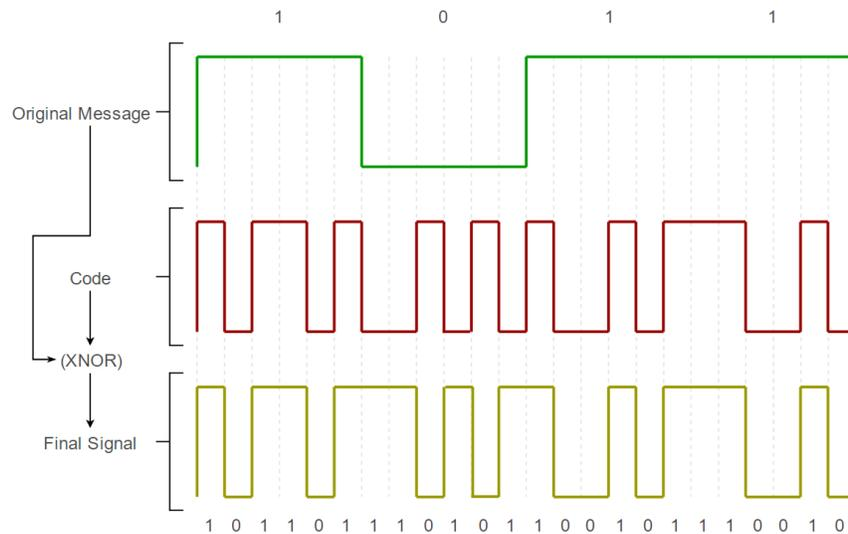
Figure 23. A CDMA approach to spreading an initial message over a greater using an example code. The original message contains four bits however the final signal is 24bits in length due to the 24bit code used.
