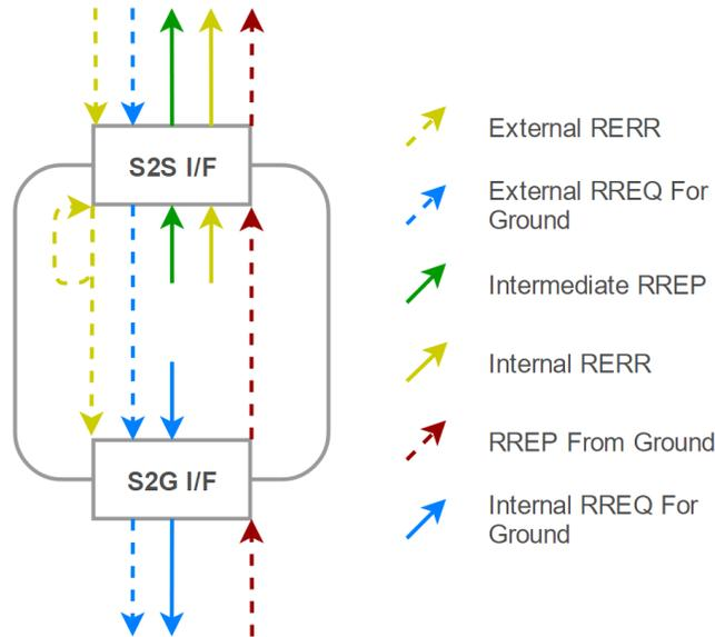
Figure 33. The interface use of a GM in response all route messages implemented by this work. In comparison, non-GMs will only ever use their S2S interfaces.
