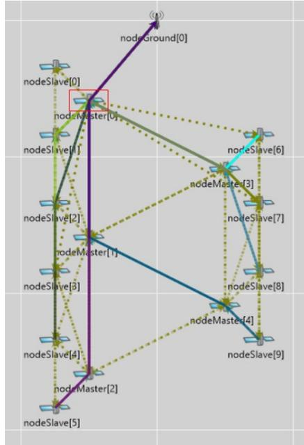
Figure 47. In CubeMac's pure TDMA mode all nodes act as masters. This arrangement creates a larger number of viable routes to ground. Solid lines above represent the movement of science data packets. This behaviour can be compared to the default CubeMac & D<sup>3</sup> behaviour as illustrated in Figure 40.
