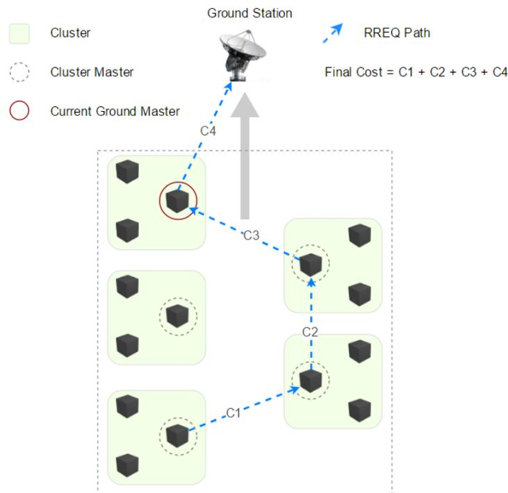
Figure 30. As an RREQ, or RREP, packet moves through a network it accumulates link costs within its 'metric' field.
