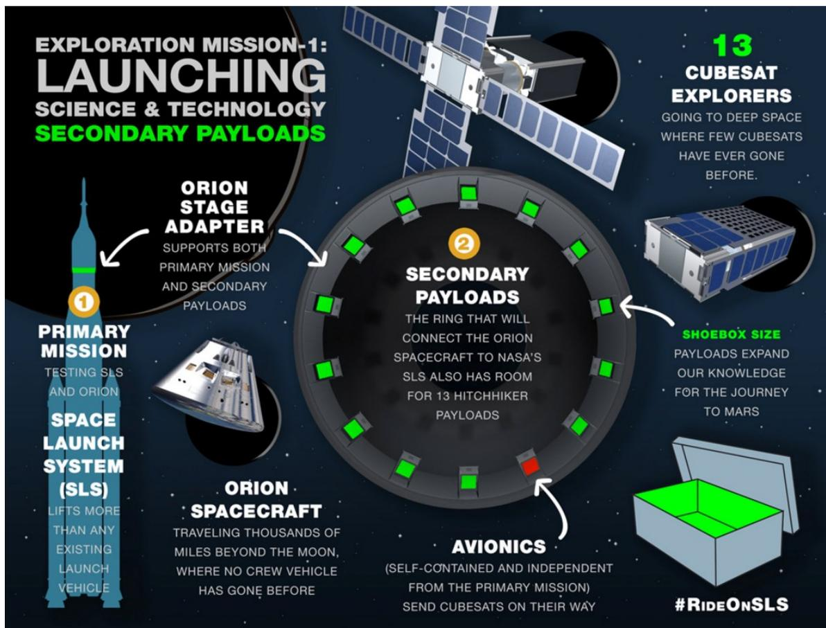
Figure 5. An illustration of the dedicated secondary payload deployers built into the “Orion Stage Adapter” of NASA’s upcoming Space Launch System. Existing launch vehicles are generally retroactively fitted with such deployers. SLS is currently projected to launch the first CubeSat into deep space in 2019. Image Credit: NASA.
