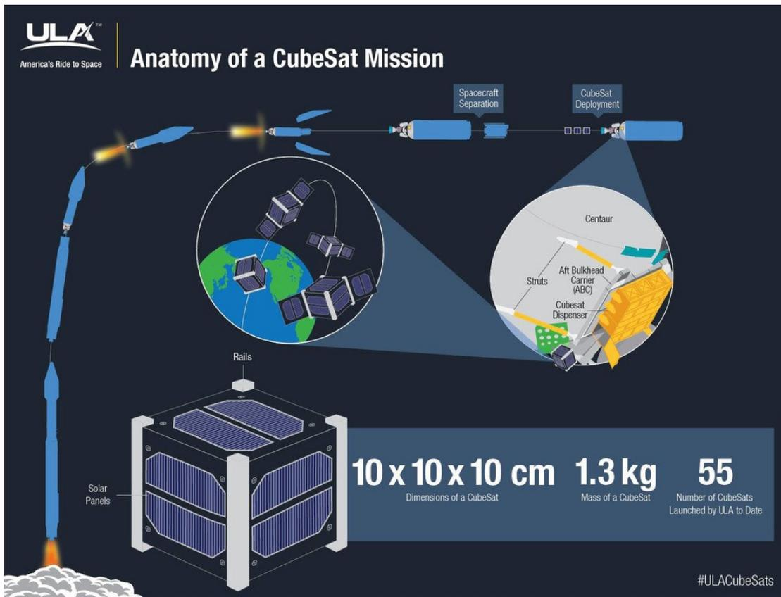
Figure 1. An illustration of the CubeSat form factor and a deployment approach. Here CubeSats are deployed prior to delivery of the primary payload using a dispenser attached to the final stage of the launch vehicle. Image Credit: United Launch Alliance LLC.
