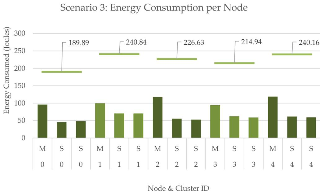
Figure 51. Due to scenario 3's altered election approach masters experience an overall drop in energy consumption when compared with scenario 1a and 2a.
