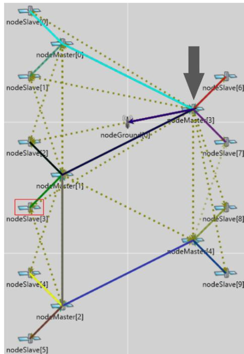
Figure 40. The closest master to ground, indicated by the grey arrow, is elected as the CSN's GM. The paths of UDP packets are indicated by solid lines. Logical routes determined opportunistically as a result of the movement of route messages are indicated by dotted lines.
