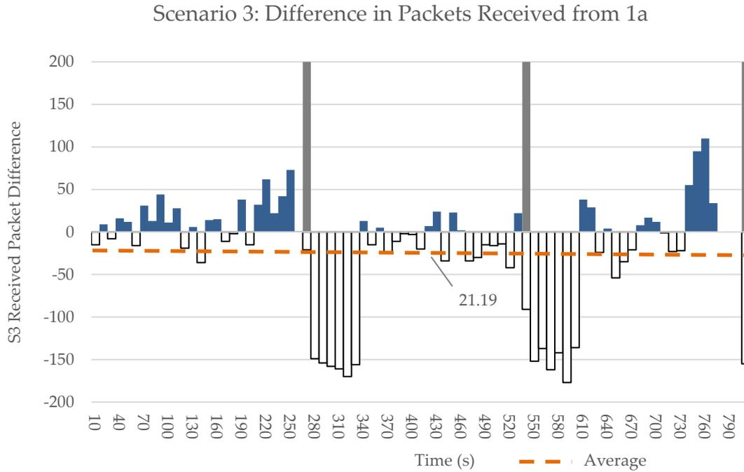
Figure 50. The difference in received packets in scenario 3 as compared with scenario 1a. Restricted ground access results in clear reductions in throughput during the opening periods of the second and third passes.
