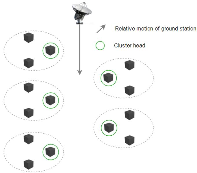
Figure 13. An example of network cluster forming and election of cluster heads. With the introduction of a mobile sink (ground station), clustering can be adapted to ensure the election of cluster heads with the longest contact durations and/or most resources [81].
