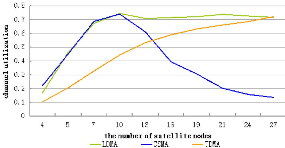
Figure 17. Cannel utilization (Vertical axis), measured from 1.0 (100%) to 0, compared to network size (Horizontal axis) for LDMA, pure CSMA and pure TDMA. Image Credit: [109]
