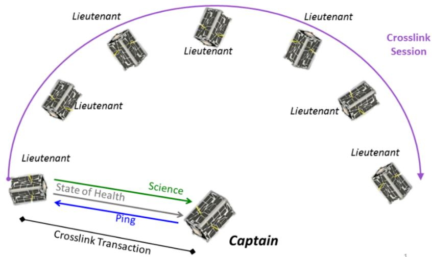
Figure 9. The Cpt/Lt protocol. EDSN designers refer to S2S communication as crosslinking. The Captain pings a Lieutenant before receiving state-of-health and science data packets. Image Credit: NASA Ames Research Centre
