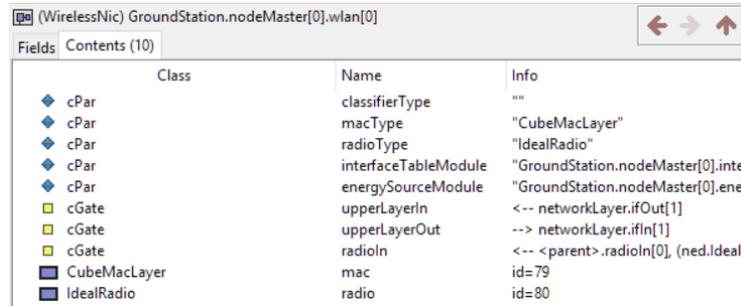
Figure 36. The parameters of and modules contained within nodeMaster[0]’s “wlan[0]” module.
