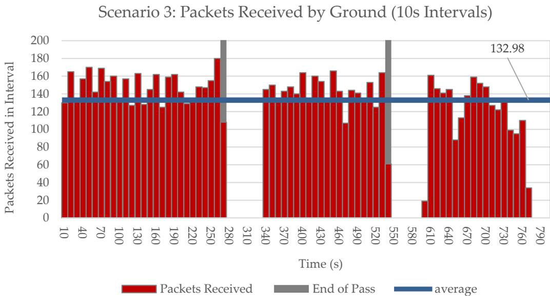
Figure 49. Scenario 3 imposes greater restrictions on access to ground through an adjusted ground master election approach. This approach results in several deliberate “gaps” in packet reception.
