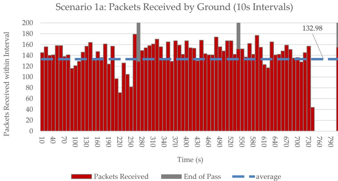
Figure 41. The number of packets received by ground station over time reduced to a granularity of ten second intervals. Each pass lasts 270s. The end of each pass is represented by a grey column.
