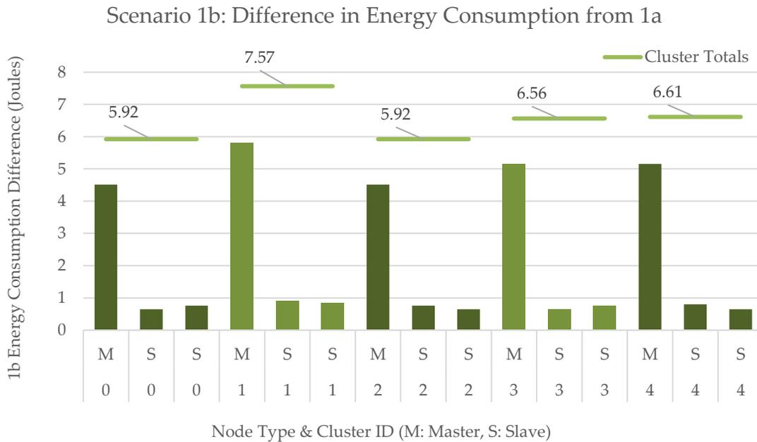
Figure 43. Energy differences calculated as the energy consumed by each node in scenario 1b less the energy consumption of corresponding nodes in scenario 1a.
