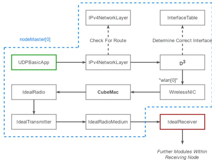
Figure 37. An example packet’s progression through various modules within nodeMaster[0] which culminates in its reception at another node within the CSN. This path represents a common progression including both D<sup>3</sup> and CubeMac.
