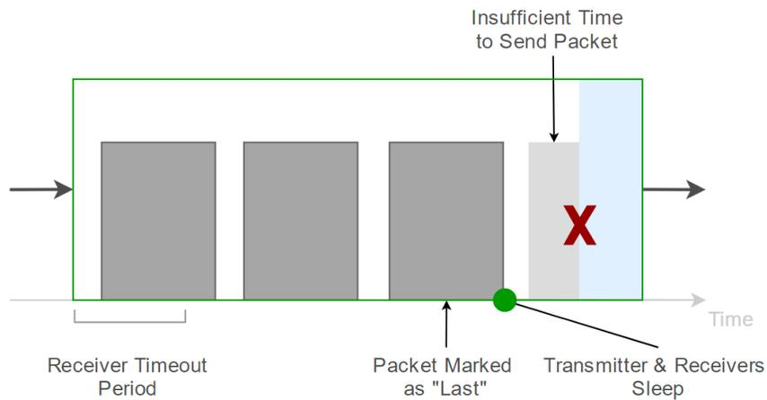
Figure 25. The last packet transmitted by any node within a time slot will contain a flag indicating that no further packets should be expected.
