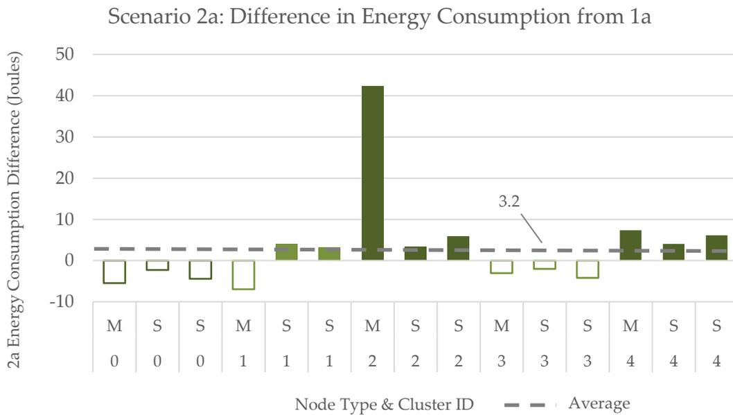
Figure 46. The change in energy consumption of individual nodes in scenario 2a as compared to scenario 1a. Negative (outlined) columns represent instances in which nodes in scenario 2a, consumed less energy overall than corresponding nodes in scenario 1a.
