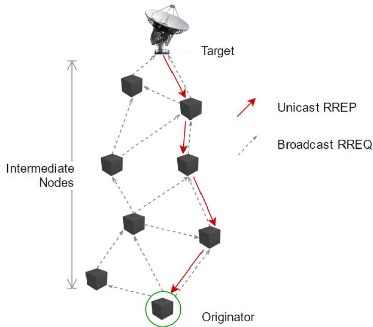
Figure 14. An illustration of the broadcast RREQ unicast RREP approaches used by DSR and AODV. Targets will generate RREPs for each arriving RREQ. RREQs which revisit nodes are dropped. The paths of dropped RREQs are not illustrated above.
