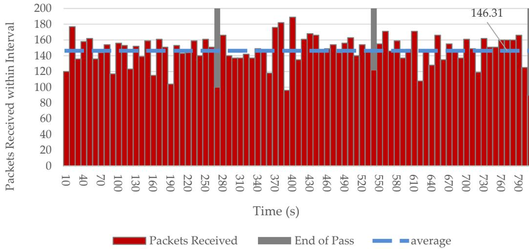
Figure 44. When compared with Figure 41 CubeMac’s pure TDMA mode can be seen to provide more consistent throughput.
