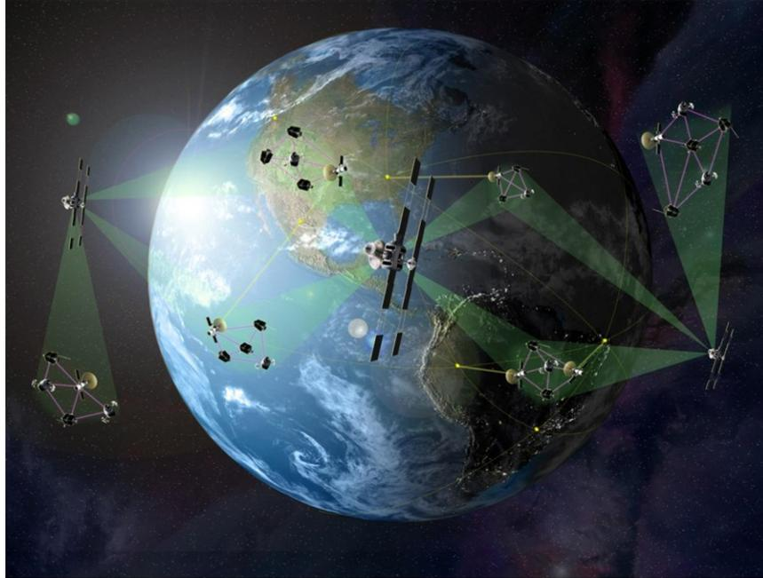
Figure 15. A rendering of the F6 DARPA fractionated satellite concept. Mission payloads exist independently of other core systems such as S2G communications. Image Credit: DARPA
