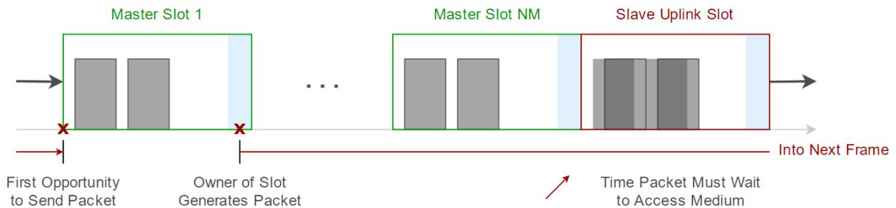
Figure 27. Packets generated within a buffer period or directly following the end of a slot must wait a minimum of approximately  $N_m$  slot durations before transmission.
