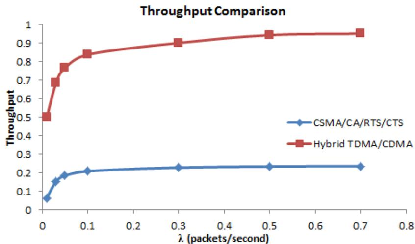
Figure 18. Throughput here is measured as the amount of time spent transmitting data divided by the amount of time available to transmit data. Image Credit: [111]
