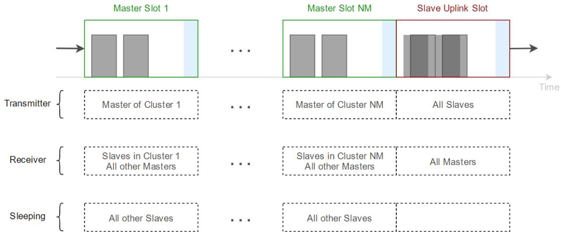
Figure 24. An illustration of the states which a given node assume during certain slots. No node may sleep during the slave uplink slot. These states are sufficient to allow multi-hop communication between all nodes within a network.
