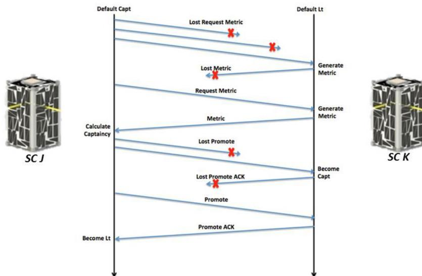
Figure 10. A timeline of the Captaincy negotiation process carried out between the two Nodes spacecraft (SC). Image Credit: NASA Ames Research Centre
