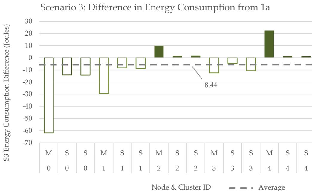
Figure 52. Negative (outlined) columns represent the energy saved by individual nodes as a result of D<sup>3</sup>'s energy-distance election approach.
