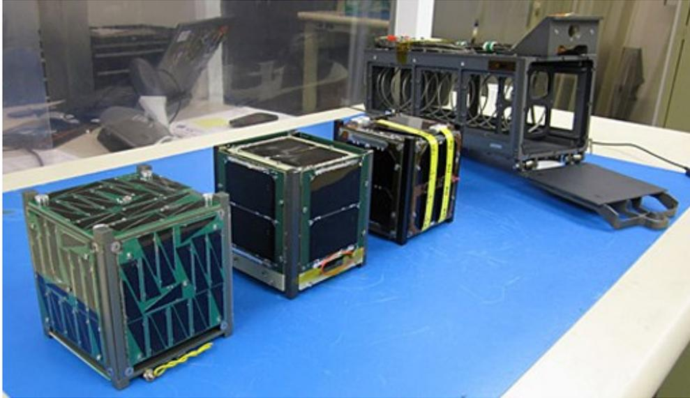
Figure 4. Three 1U CubeSats beside a 3U (Poly Picosatellite Orbital Deployer (P-POD) developed at CalPoly. The spring mechanism used by P-PODs to deploy CubeSats can be seen within the main housing. Image Credit: California Polytechnic State University
