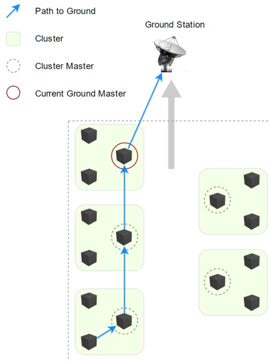
Figure 22. All routes from slaves to ground require one or more masters. The Ground Master always constitutes the final hop on a path to ground.
