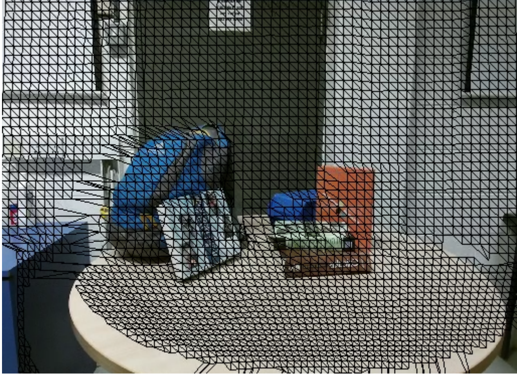
FIGURE 4.5: Triangle mesh rendered in top of the color image. The triangle mesh match the real world image by the transformation of the view and projection matrices.
