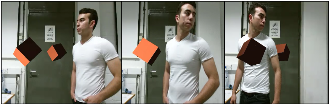
FIGURE 5.1: Frame sequence of the user occluding one virtual object in the scene.
