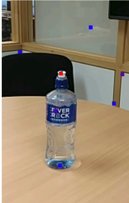
Figure 21 - Tracked feature points being drawn on screen in debug mode of android application as small multi-coloured rectangles.
