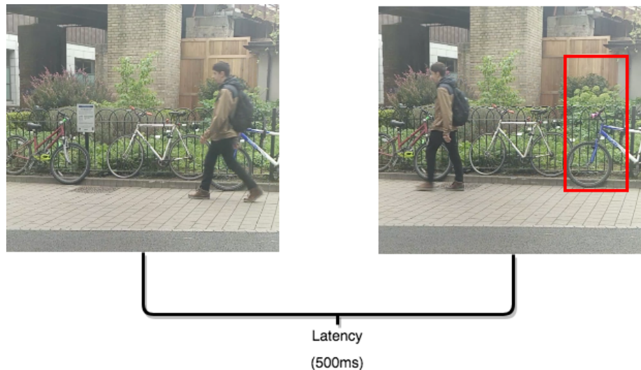
Figure 16 - Stale frame due to latency of object detection.
