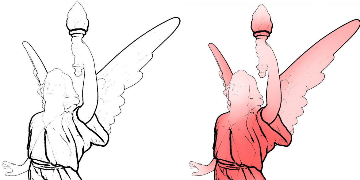
Figure 17 Left: variable line thickness rendered over with white. Right: illustrating the red channel of the vertex colours.
