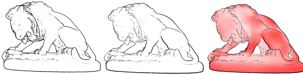
Figure 20 Left: constant vertex extrusion. Centre: variable vertex extrusion. Right: illustration of vertex colours. This model was obtained from https://sketchfab.com/models/d5e6b6a11da646f68a5fcba661dcae99
