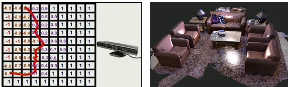
Figure 2.5: a) Example of a 3D-reconstructed scene with Kinect Fusion [46]. b) Truncated signed-distance function using a Kinect as scanning device [17].
