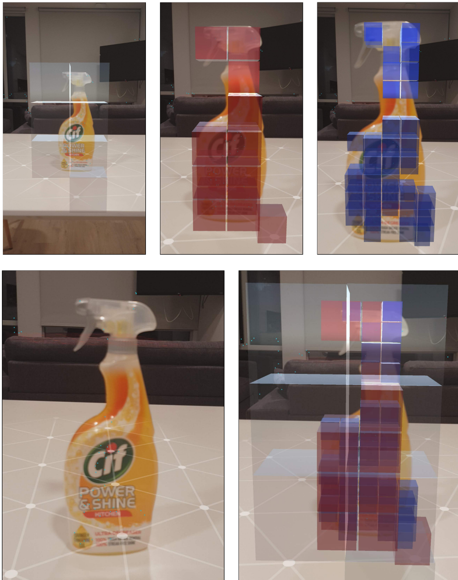
Figure 6.2: a) Level of detail 0 with 10\text{cm}^3 voxels. b) Level of detail 1 with 5\text{cm}^3 voxels. c) Level of detail 2 with 2.5\text{cm}^3 voxels. d) Real object with only a plane being rendered. e) All resolutions rendered simultaneously.
