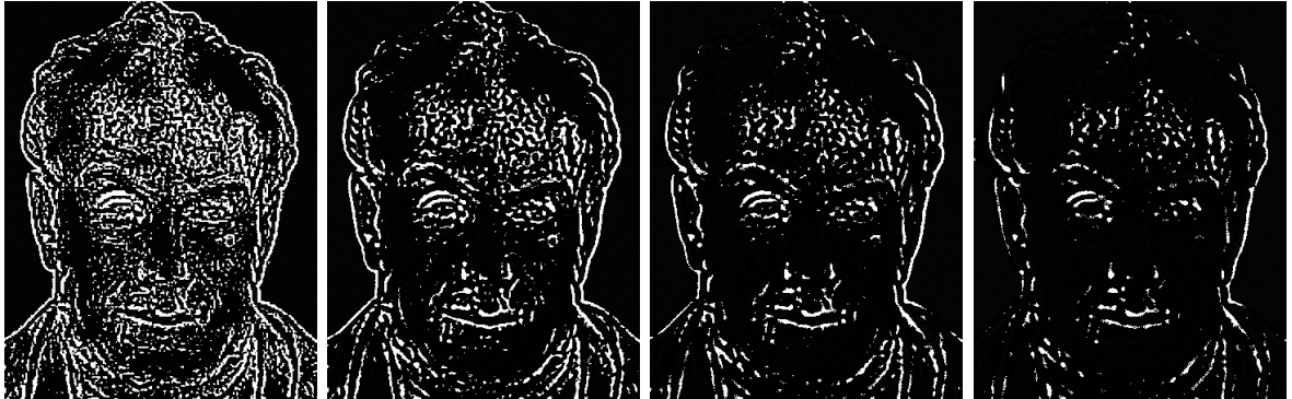
Figure 2.5: Approximating Laplacian of Gaussian using the Difference of Gaussian method on the first octave
