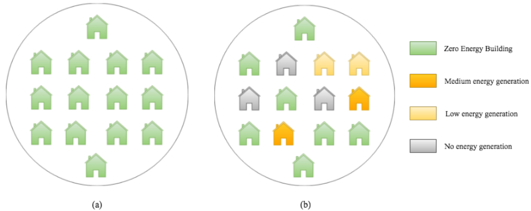
Figure 1.1: (a) A nZEC community consisting of only nZEBs. (b) A nZEC community having buildings with varying generation capacity.
