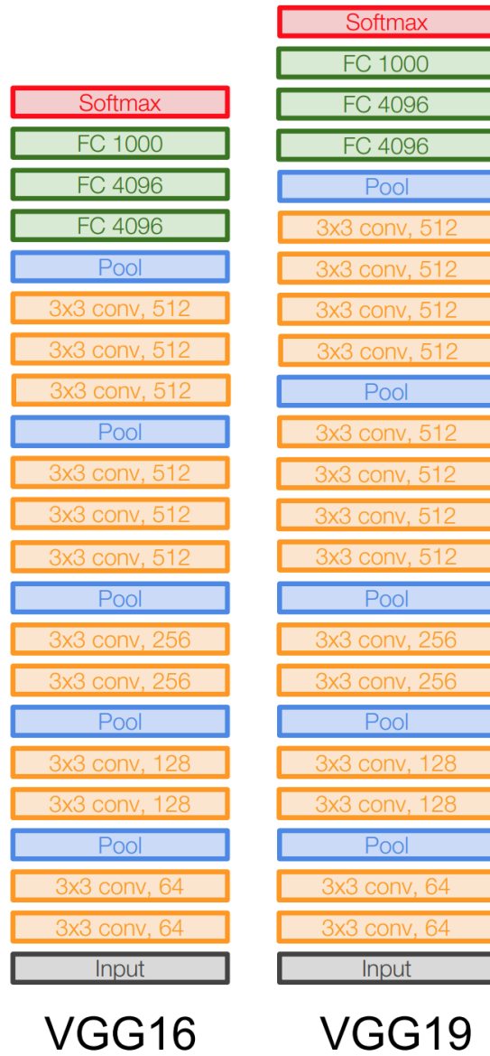
Figure 3.3: VGGNet Overview: Strictly use 3 \times 3 filters with 2 \times 2 max-pooling layers [36].
