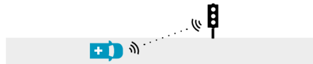
Figure 10: PVD example, sensor data from passing traffic is collected for use by traffic management (BMVIT, 2016)
